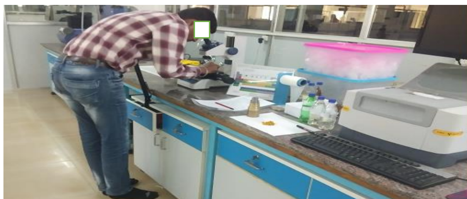
Fig. 3(a). The MITUTOYO microscope and X-Ray Fluorescence Spectrometer (XRF) to take a microscopic view and the elements in Turmeric of various varieties (CUTM Lab, BBSR)
